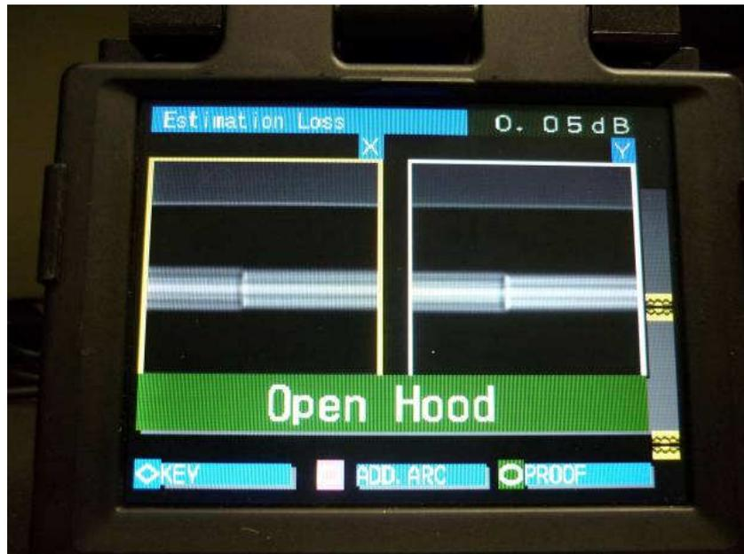
**Draka BendBright XS spliced to BendBright Elite (Trench Assisted G657A2 to G657B3)**
