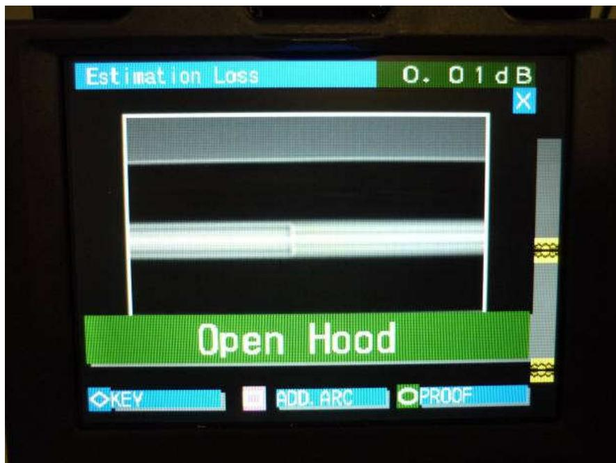
**Draka BendBright Elite (Trench assisted type G657B3 ) spliced to G652**
