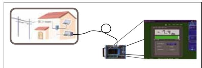
Fig. 4. Optical power monitoring at the FTTx end-user side
