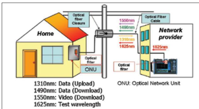
Fig. 7. Using the 1625nm wavelength for surveillance of an active optical network
