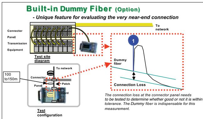
Fig.2. Built-in Dummy fiber for evaluating near-end connection
