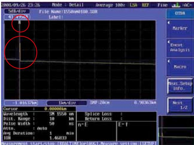
Fig. 3. Display of measurements made using built-in Dummy Fiber; different colours are used to distinguish the waveforms from the Dummy Fiber and the measured Fiber
