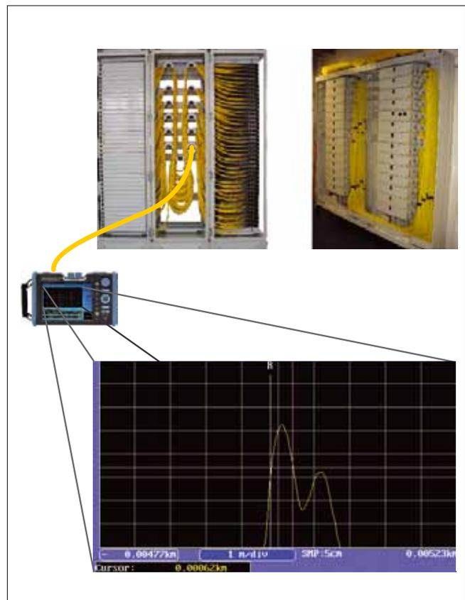
Figure. 1. Waveform display showing ODF measurement using 0.8 m dead zone
