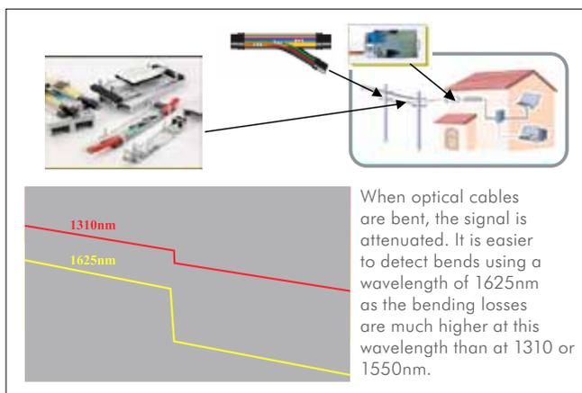
Fig. 6 Using the 1625nm wavelength to detect bending losses
